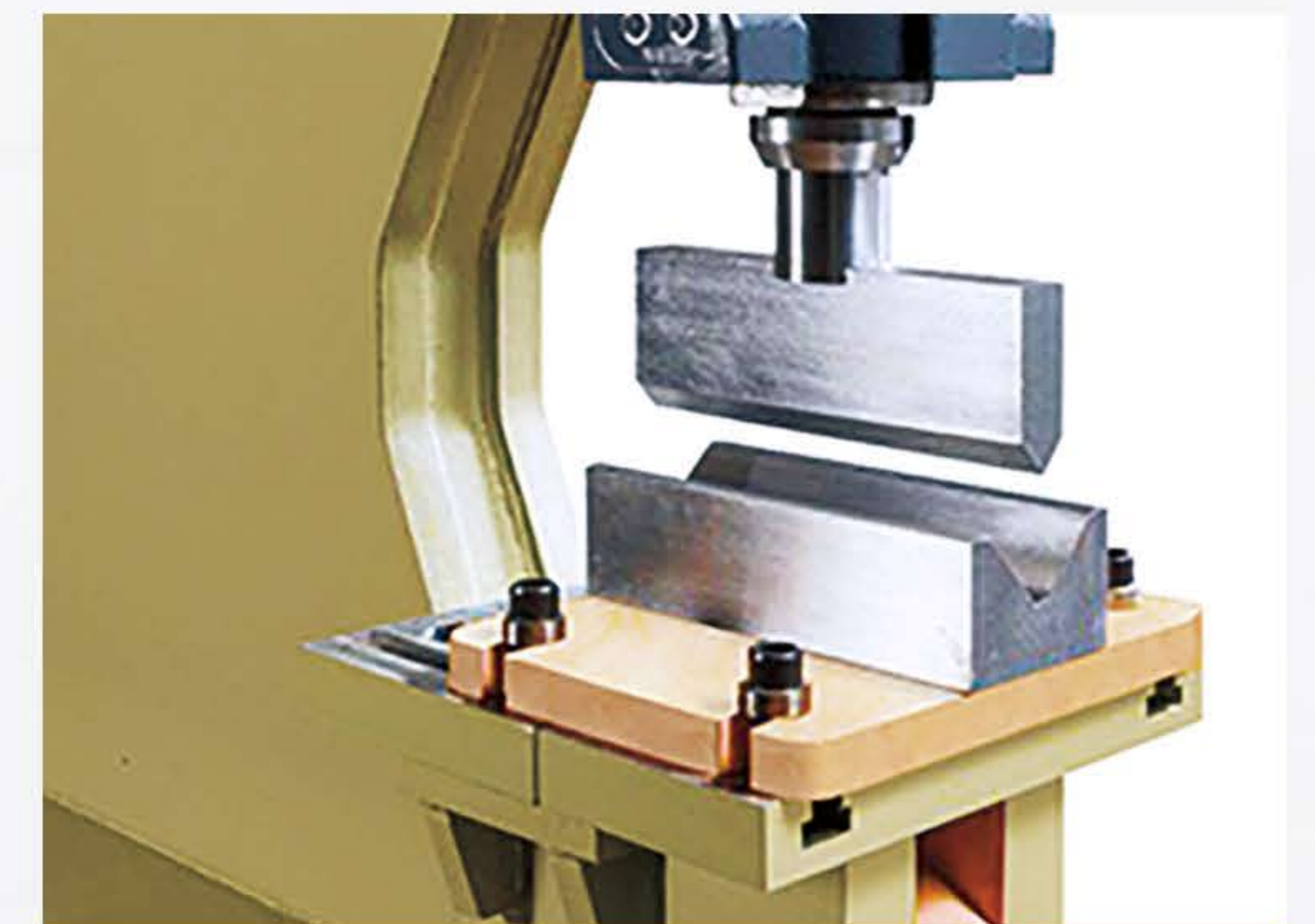
Lengthwise Installation Of Bending Die
